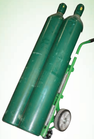
Mag-2 Height: 53" Width: 19" Weight: 116 lb. Wheels: SC-33, R3 Cylinder capacity: 9.5"
