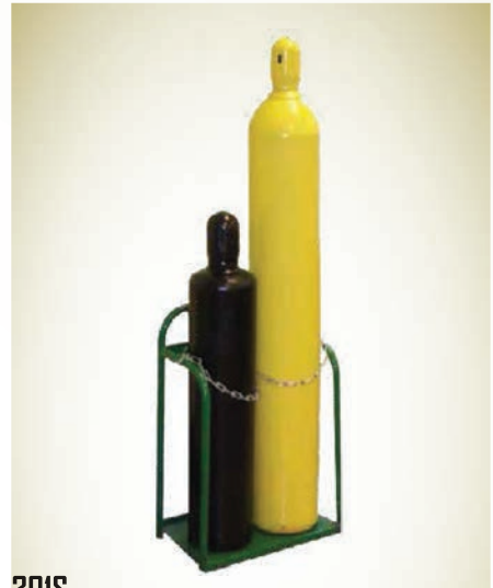
301S Baseplate: 21"x12" Height: 29" Width: 21" Weight: 20 lb. Cylinder capacity: 9.5", 9.5"
