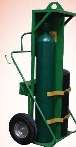
552-16H-FW Baseplate: 13" x 24" Height: 78" Width: 35" Weight: 196 lb. Wheels: SC-11B Cylinder capacity: 9.5" , 12.5"
