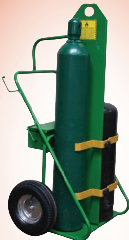
552-16FW Baseplate: 13" x 24" Height: 65" Width: 36" Weight: 130 lb. Wheels: SC-11B Cylinder capacity: 9.5" , 12.5"
