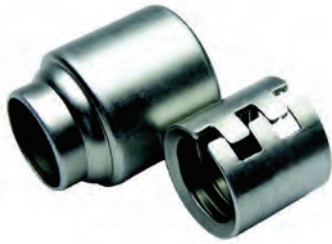
During crimping, only the MegaCrimp coupling's outside shell takes on the shape of the dies. The "C" insert starts round, stays round – like the hose.
